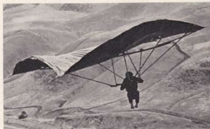
(Above and below) An early basic bamboo-and-plastic Rogallo glider. The pilot literally hangs from the framework below the sail. (Bottom) A more modern Rogallo with a swing seat.
