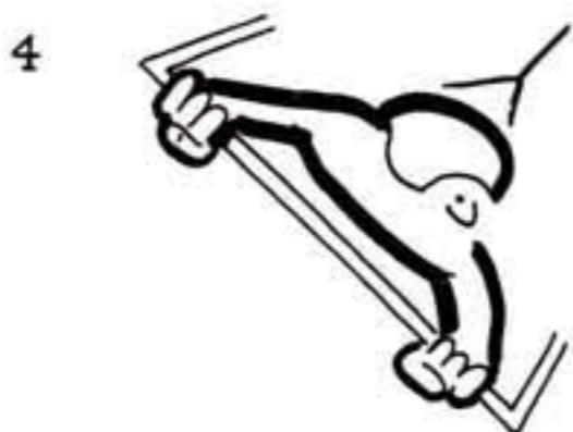
Control rate of turn by pitch movement on bar: both arms NOTE: pilot now almost central on bar; but still looking into turn.
