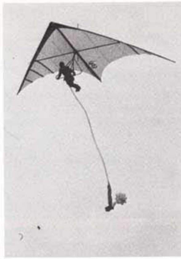
Top left: Canopy falls away from glider. Drogue deploys prior to strop breaking loose attachment points. Above right: The instant of deployment. The canopy is almost horizontal to the glider flight path and is acting as an effective airbrake. Tony instinctively pulls on speed to counteract the slowing effect. Right: The glider starts a gentle swing to hang vertically below the canopy.
