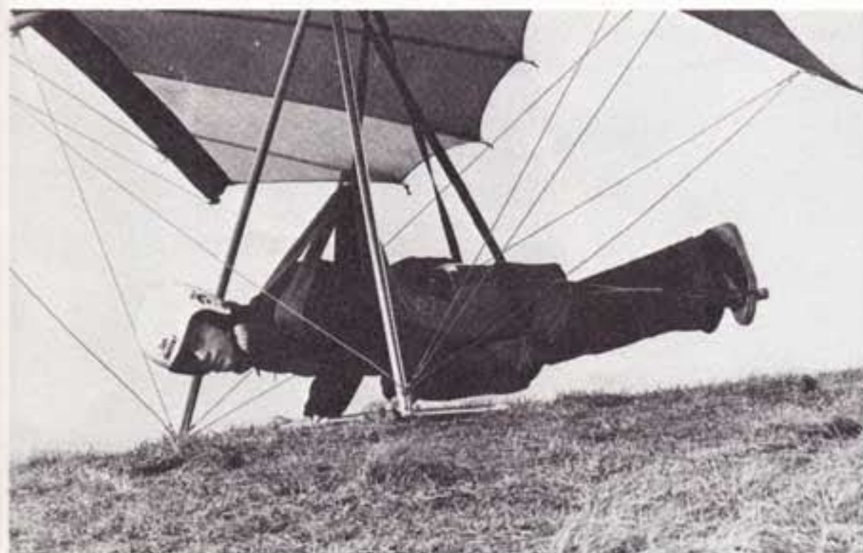
When flying prone, the packed parachute must clear bottom bar
